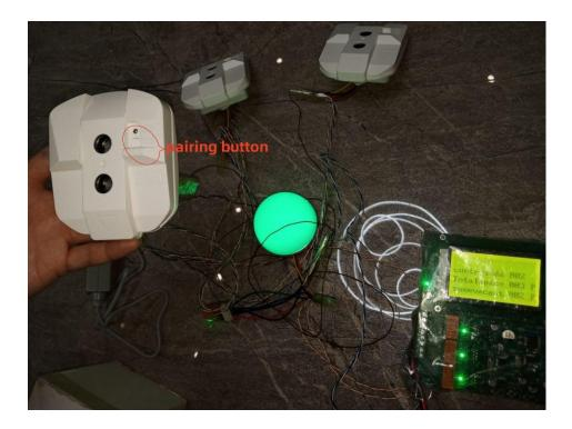
For example in the above picture as refer area controller is 001 address ,detector set up address is 20
