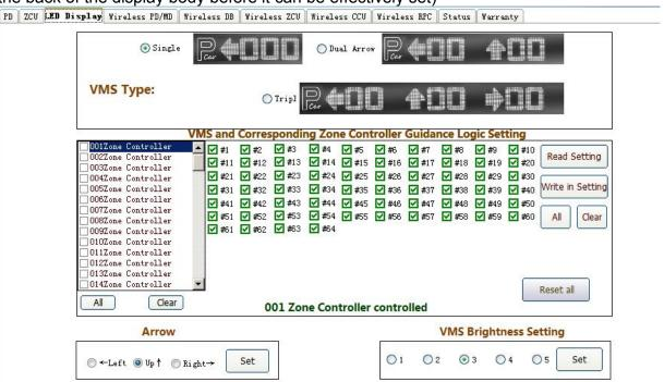
Install and open the parking tool debug software choose the controller and the paring detector will display out for doing the linkage
